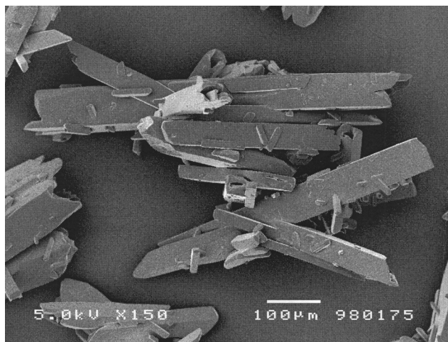
Figure 4. Monohydrus sodium carbonate, crystallized with ethylene glycol, x_{EG} = 0.67 at 90^{\circ}\text{C} .
